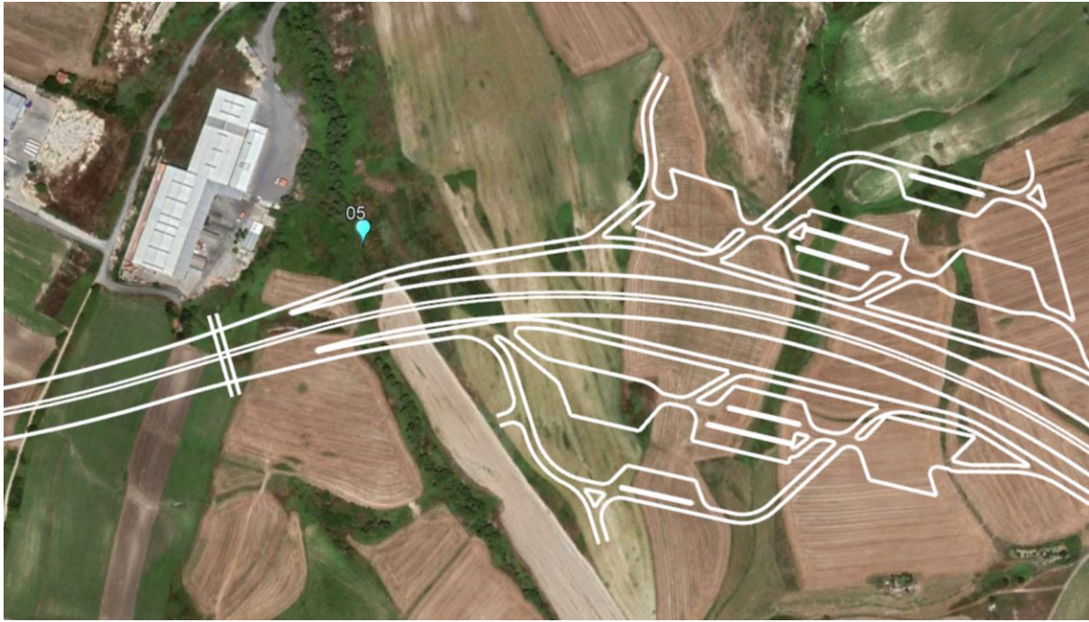
Figure 15. Satellite image of the study point 5. White line is the Motorway route planned.
